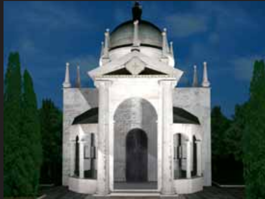
External lighting: 2100 Medio Floodlight HQI-G12 70W with etched glass and 2x17° optics (code 82 30 111)
