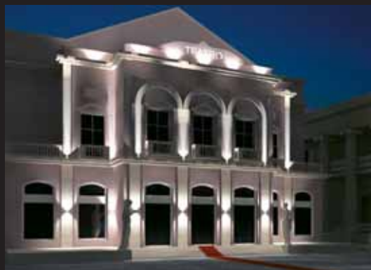
Tetra Applique 140 2xHQI-G12 35W (code 50 20 622) and Tetra Applique 140 1xHQI-G12 35W (code 50 20 612) with 2x16.2° optics
